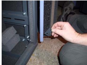
3. Offer up the second fixing plate to bottom bracket
