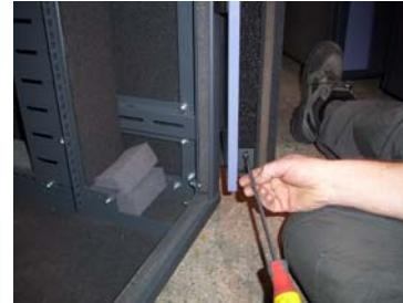
4. Fix in place with the other fixing plate – then repeat process on the other door
