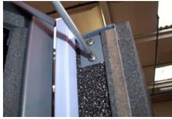
1. Place the foam at the top bracket on the inside of the front door side – fix into place with one of the fixing plates and secure.
